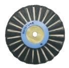
The Calico Interleaved Lathe Brush is a diverse 3-1/8" dia. polishing brush. It has three rows of converging bristles and two rows of Muslin buffs. The bristle is made of Chung King bristle with Muslin buff interwoven. This item is long lasting and saves time and labor. It polishes much faster than the standard brush.
