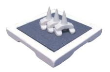
These Carbon Insert Ceramic Trays absorb silver vapor that is released during each firing. It's a must-use with silver palladium alloys. Items also come with 6 anterior pegs or 6 carbon replacements. Size: 2-1/4" x 2-1/4" x 1/4" (57.1 x 57.1 x 6.3 mm).
