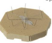
The Keystone Spider Tray is a new firing tray utilizing a fixed fan shaped pin specifically developed for all types of delicate ceramic work with an emphasis on all-ceramic restorations. With 8 bendable, thin metal prongs, the tray can adapt to a variety of cases. The unique shape and thinness of the blades allow a more uniform cooling of the ceramic restoration.
