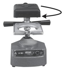
5. Swing the heating unit into position directly over the material.
