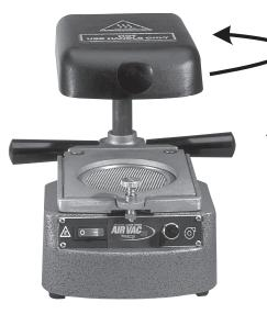
1. Swing the heating handle unit to the rear and turn on the heating element switch. It will require approximately one minute to preheat. Preheating the unit before use is especially important when using materials .040 or thinner. These materials heat very quickly and it is best to have the heater temperature stabilized first.
