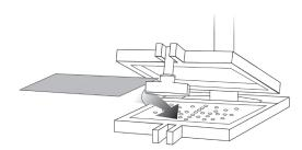
2. Open the hinged frame by turning the latch knob. Place a sheet of forming material on the lower material plate. Lower the top material plate over the material and engage latch.
