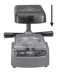
7. Turn off the heater switch and turn on the vacuum pump switch to complete the adaptation (approximately 15 seconds). Most forming takes place immediately however with thicker materials, allow the pump to run longer for finer detail.
