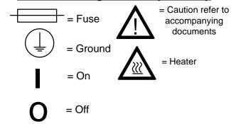
Fuse Replacement: 240 volt(Max) 1 Post - 6.3A 250V 120 volt 1 Post - 15A 125V
