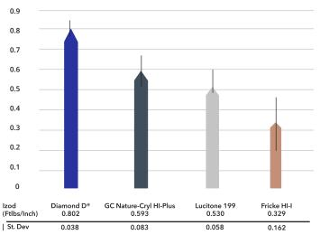
Source: Notched Izod Impact Strength Determinations per ASTM D256. Submitted in ASTM D638, Type 1 specimen form. Performed at Bodycote Polymer-Broutman Laboratory, a UL and IAPMO approved independent testing laboratory, A2LA and IAS sccredited. BBI Test Reference #s: 30002570 and 30000666.
