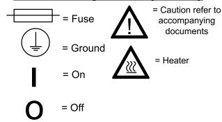
Fuse Replacement: 240 volt(Max) 1 Post - 6.3A 250V 115 volt 1 Post - 15A 125V
