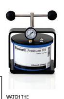
Bosworth's Pressure Pot is a hydraulic water press used in creating bubble-free relines, repairs, splints, temporaries, and orthodontic appliances. It guarantees a dense, super smooth, porosity-free surface on any self-curing acrylic with just 10-15 p.s.i. Create a temporary with Pressure Pot to increase strength by reducing voids and porosity. Pressure Pot does not require electricity, heat, or air pressure. It is lightweight and easily transportable.
