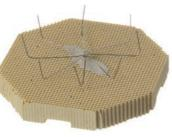
The Keystone Spider Tray is a new firing tray utilizing a fixed fan shaped pin specifically developed for all types of delicate ceramic work with an emphasis on all-ceramic restorations. With 8 bendable, thin metal prongs, the tray can adapt to a variety of cases. The unique shape and thinness of the blades allow a more uniform cooling of the ceramic restoration.
