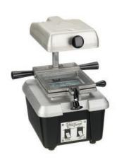
The Single Chambered Vacuum Former is an economical answer that can still excellently fabricate most thermo-plastic appliances. The all-aluminum construction eliminates rusting and the heating element is symmetrically engineered for uniform heat distribution. The hexagonal post keeps the frame from rotating or sliding. This vacuum former uses 5" x 5" (12.7 x 12.7 cm) resin sheets. Made in the USA.
