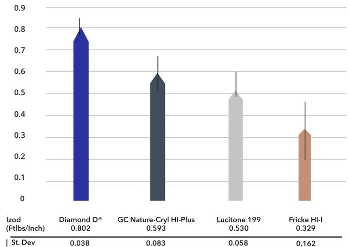
Source: Notched Izod Impact Strength Determinations per ASTM D256. Submitted in ASTM D638, Type 1 specimen form. Performed at Bodycote Polymer-Broutman Laboratory, a UL and IAPMO approved independent testing laboratory, A2LA and IAS accredited. BBI Test Reference #: 30002570 and 30000666.
